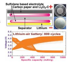
By optimizing the battery formula, including solvents, salts, current collector, and positive electrode materials, a lithiumair battery can operate 800 cycles with a specific capacity of 1000 mAh g<sup>-1</sup>. The findings described here are expected to benefit the pursuit of green, sustainable, and high-performance lithium-air batteries.
