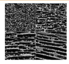
Bioinspired scaffolds with equal porosity, but different pore architectures exhibit compressive mechanical properties that change as a function of the pore morphology. The scaffolds are fabricated by freeze casting with different soluble additives to alter the viscosity, pH, or alcohol concentration. A simplified Euler buckling analysis predicts the strength of the scaffolds as a function of the pore aspect
