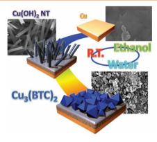
HKUST-1 [Cu<sub>3</sub>(BTC)<sub>2</sub>] coatings a good adhesion are homogeneously fabricated on copper metal plates, 3D objects, and patterns. The metal organicframeworks (MOFs) are converted from any metallic Cu object via Cu(OH)<sub>2</sub> nanotubes at room temperature in approximately 30 min using an aqueous ethanolic mixture. The conversion mechanism from copper hydroxide nanotubes into Cu<sub>3</sub>(BTC)<sub>2</sub> is revealed by electron microscopy time-course monitoring.
