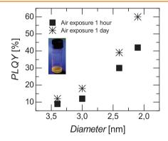
ZnO quantum dots are prepared in a nonthermal plasma reactor operated with a high frequency source. Quantum dots with diameters down to 2.1 nm are achieved, exhibiting exceptional high quantum yields up to 60%. The mechanism for the dominating green-yellow emission is discussed and the influence of oxygen species on the emission spectrum is investigated.
