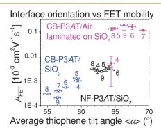
The orientation and organization of semiconducting polymer at the polymer/(gate dielectric) interface has a strong influence on OFET hole mobilities. For poly(3alkylthiophene) thin films, both from chlorobenzene and from nanofiber dispersions, orientation and OFET mobility are compared for the interfaces formed at bare SiO2 and at air (then laminated on bare SiO<sub>2</sub>), that is, at two extremes of the polarity scale.
