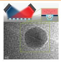
Materials libraries of Au-Cu alloy nanoparticles (NPs) synthesized by combinatorial co-sputter deposition of Cu and Au into the ionic liquid (IL)  $[C_1C_4im][Tf_2N]$ are investigated by TEM, XRD, UV-Vis, and ATR-FTIR spectroscopy. A new NP isolation process is developed enabling separation of NPs from IL without changing size, morphology, composition, and aggregation state.
